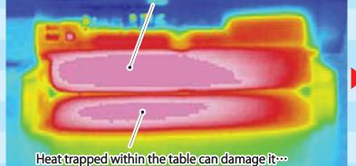
Heat transferred to the table is trapped, causing a reduction in cooling efficiency, and resulting in further load on the game console.
